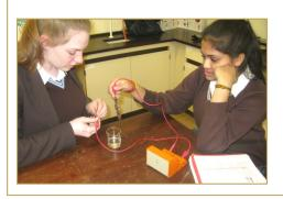
They set up their apparatus and used it to investigate the voltage produced by different metals. They were interested to discover that you can make a voltage with
